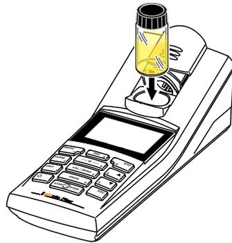
**Inserting a 16 mm cell**
